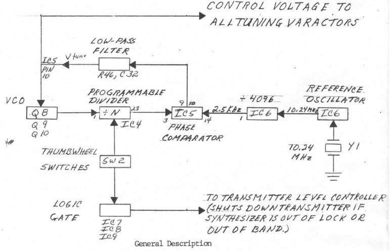
The output of a stable reference oscillator, and the output of a voltage-controlled-self-excited oscillator, are fed to a phase comparator. A DC error voltage is derived, from the phase comparison, that is fed back as a control voltage to the VCO in a manner that will cause the two frequencies to synchronize. The error voltage is also used as a tuning control voltage for the varactor diodes in the receiver and exciter.
